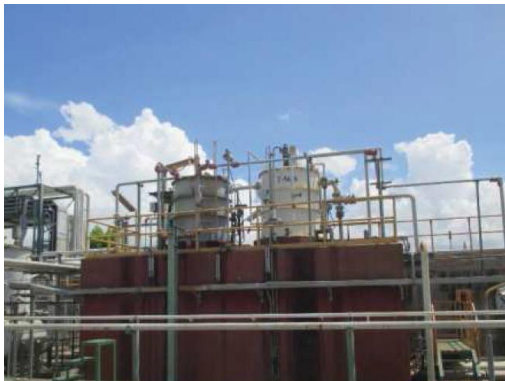
Neutralization Tank
